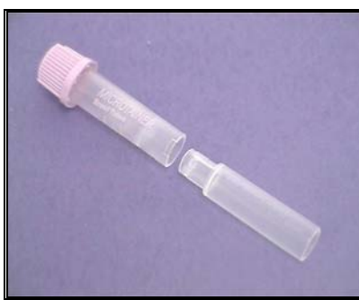
BD Microtainer Lavender Top 500 \mu L Plastic Tube (K 2 EDTA) with Microtainer Tube Extender
