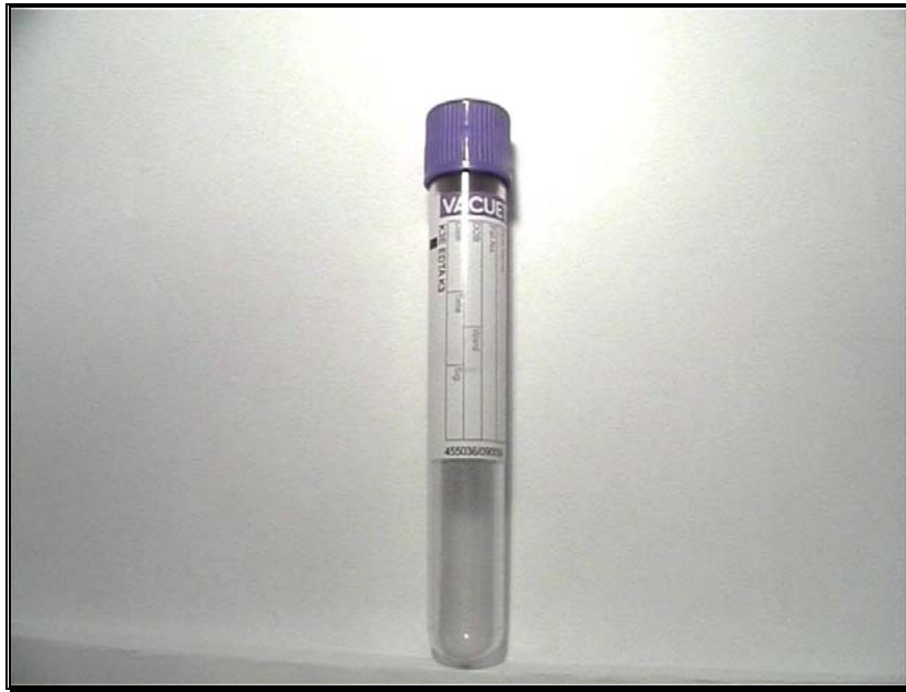
Greiner Vacuette Lavender Top 9.0 mL Plastic Tube 1.8 mg K 3 EDTA
